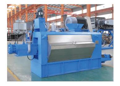
Sensitar Oil Press provides highly effective mechanical extraction of the fat content from cooked and dried animal and poultry by-products, in a continuous flow. This enables you to achieve a hard cake with a low fat content.
