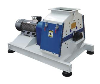
Milling Plant effectively reduces the size of particles in the not-yet-finished meal after fat extraction, helping you meet customer specifications about particle size.
