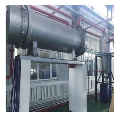
When the temperature of the two different fluid from tube wall flow heat exchanger channels on both sides, the two counter-current touch fluid through the pipe wall. Heat is by the thermal fluid flow to the pipe wall, and then from the wall to cold fluid, so as to achieve the high temperature gas into tasteless condensate purpose at low t emperature
