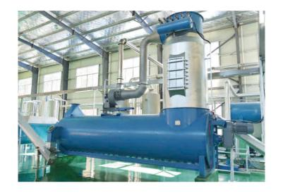
Sensitar Cooler adopts rapid flow type to cool powder and small granular materials.
